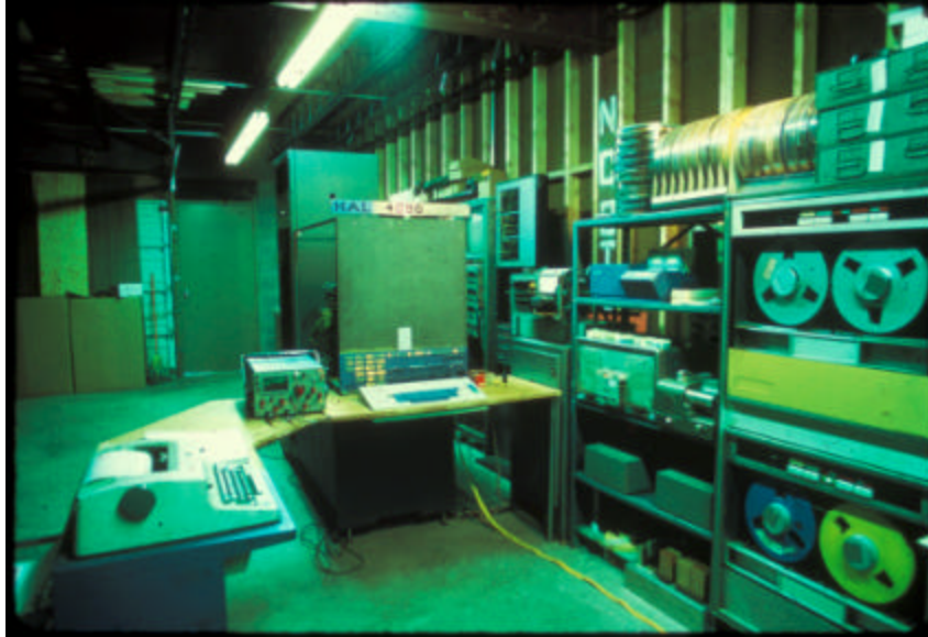
1970 – Hal Chamberlin's computer built from obsolete parts and his own design processor with 4KB of RAM
