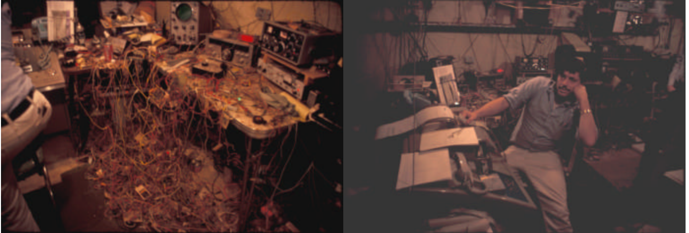
1973 –8-bit Computer built by Roger Amidon using TTL integrated circuits.
