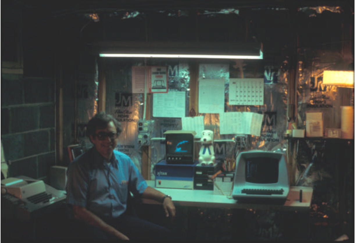
1977 – Sol Libes & his Z-80-based system running CPM. Dual floppy disk drives CRT terminal and graphics display.
